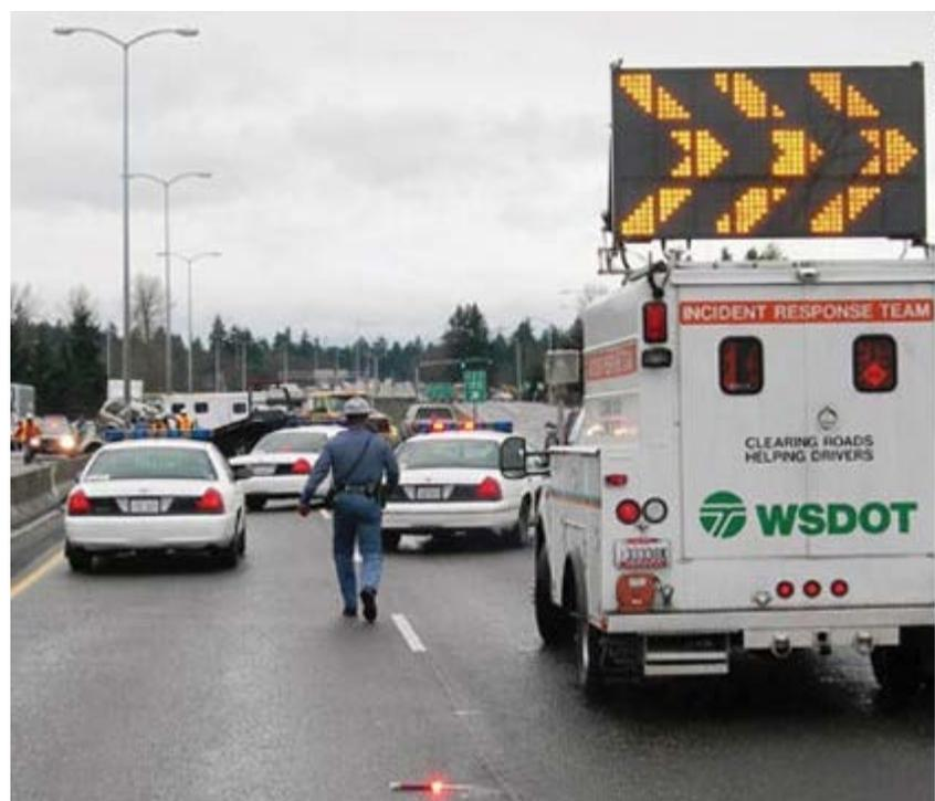
WSDOT's Incident Response Team is assisting State troopers and other responders working to clear an incident. The electronic sign mounted on top of the truck helps to redirect traffic around the scene of the crash. (Note: FHWA endorses the use of high-visibility vests by every responder.)
