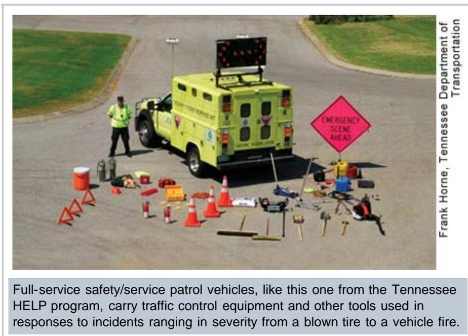
Full-service safety/service patrol vehicles, like this one from the Tennessee HELP program, carry traffic control equipment and other tools used in responses to incidents ranging in severity from a blown tire to a vehicle fire.
